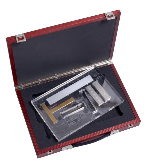
Smaller, simpler CR Phantom for Qualification of CR Systems Process Control and Long-Term-Stability
